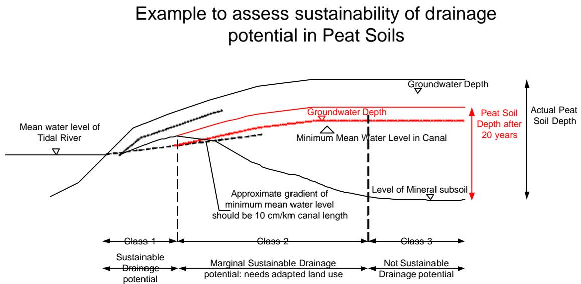
Because the actual drainage potential might not be sustainable for the future the Balance/Duflow/Modflow modeling should be repeated based on the expected subsidence of the peat layers at respectively 10 years, 20 years and 40 years after reclamation. This computer modeling will provide the best estimates for the sustainability of the present or proposed land use on the ombrogenous peat domes.
