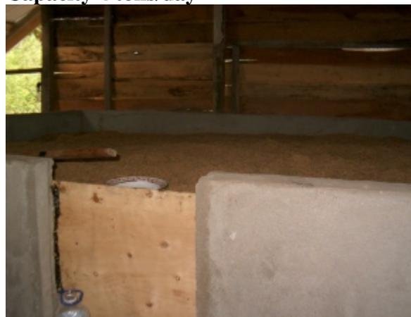
The box-drier using husks is as efficient as the box-drier using kerosene. (No costs and there are not more husks needed than will be dried by the burning.)
